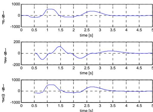
Fig. 13. Response time model - working stroke of 50 mm
