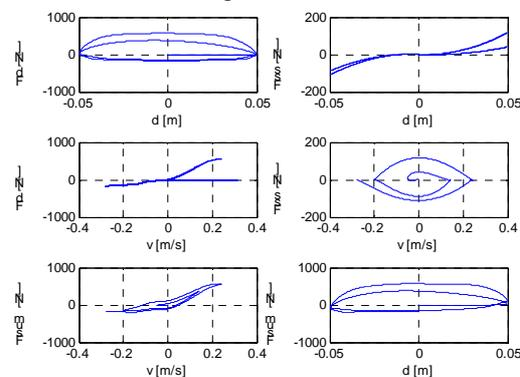
Fig. 14. Simulation results - 50 mm stroke force
